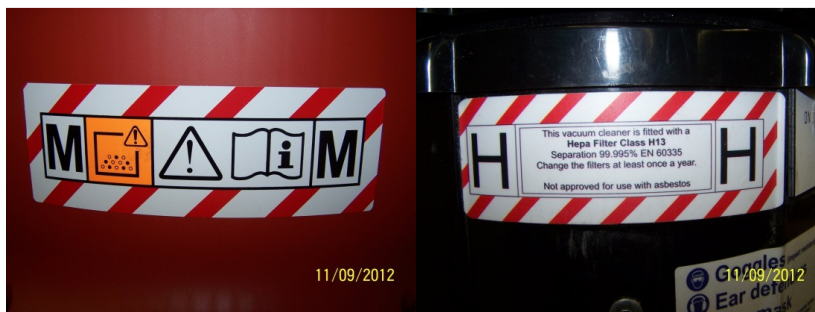
Figure 4 Label on M and H class extraction units (Source HSE, GB)
